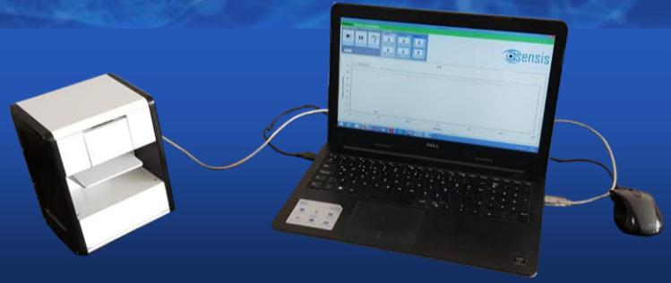
**QTF F-Master** is the first fully integrated QTF based mass sensitive biosensor measurement system. It consist of QTF driver circuit, frequency counter, vertical liquid alignment system and F-Master software. It is used via computer over the USB cable. The system does not require any adjustment or any setting. It is complete and ready to use. As soon as you plug the power and USB cable you are ready to make experiment.
